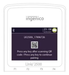
**Step 5.** Use your POS to finish Bluetooth pairing. You will see a confirmation code on the POS and the Link 2500. Once you have confirmed they match you <u>MUST</u> confirm to connect on both the POS and the link 2500 by pressing the green button. Starting with the POS and then the Link 2500.
